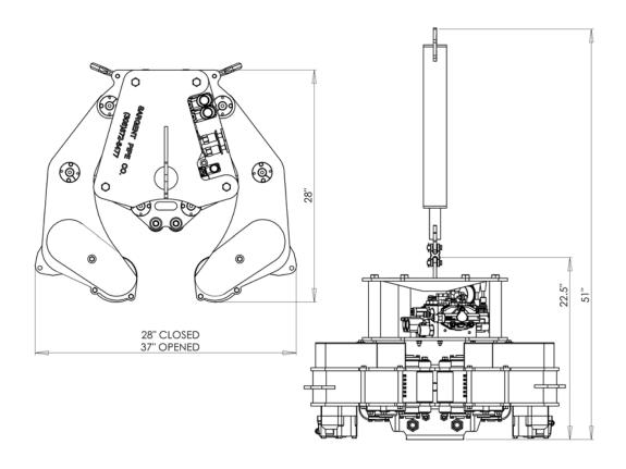
THEORETICAL TORQUE 3000PSI @ 25 GPM 10" PIPE 2295 FOOT POUND OF TORQUE @ 90 RPM TORQUE CHART ON NEXT PAGE
